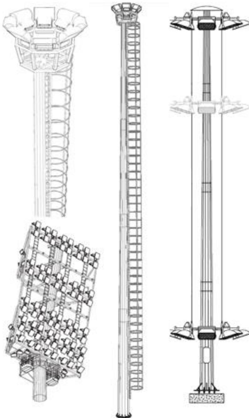
In telescopic high mast light tower, the ascending and descending mechanism for the projector basket is designed in such a way with parts to enjoy maxim safety and security. Double gearbox motor, control circuit with valid parts from valid manufacturers, automatic interlock system etc. have been designed and manufactured.
