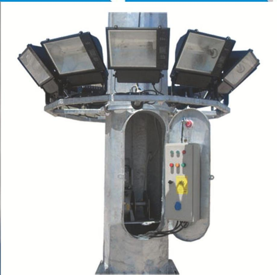
These towers are usually 12-30 m high in the motor and motorless types with fixed and moving baskets. Their external surface is protected using hot galvanized steel and their parts are assembled in the overlap form. Their basket security is supplied via interlocks and parachutes.
